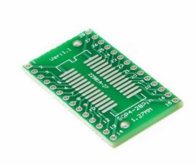
TSSOP28 SOP28 SMD to DIP28 IC Adapter Converter Socket Board Module Adapters Plate 0.65mm 1.27mm Integrate
