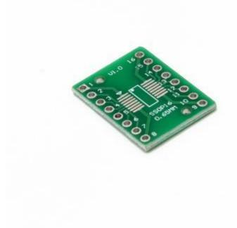
TSSOP16 SOP16 SOP16 SMD to DIP16 IC Adapter Converter Socket Board Module Adapters Plate 0.65mm 1.27mm Integrate
