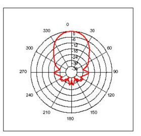
Beam Spread @ 40kHz (-6dB)
