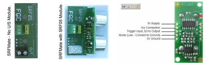
SRFMate makes connection easier and also allows 'daisy-chaining' of 5V/Gnd power supply.
