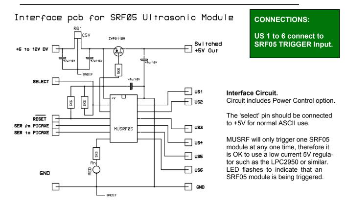
Both Serial connections (to & from Basic Stamp / PICAXE) must use 2K2 resistors to limit current.
